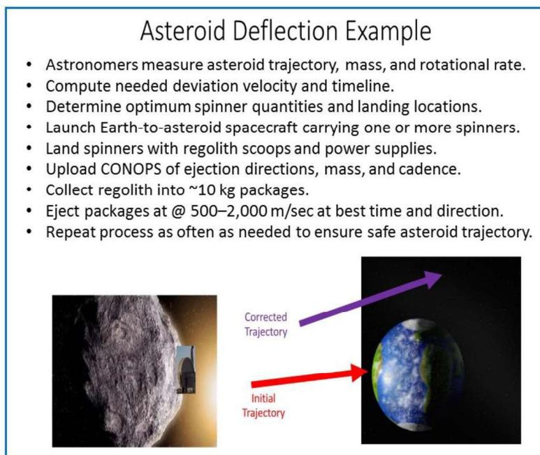
Figure 1. Asteroid deflection concept using a spinner(s).
