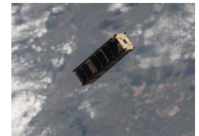
EntrySat 3U CubeSat, deployed from the ISS in 2019 (ISAE-SUPAERO)
