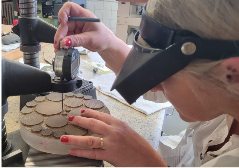
Figure 4: Thickness measurement of one pair of plates during the grinding and wedging process.
