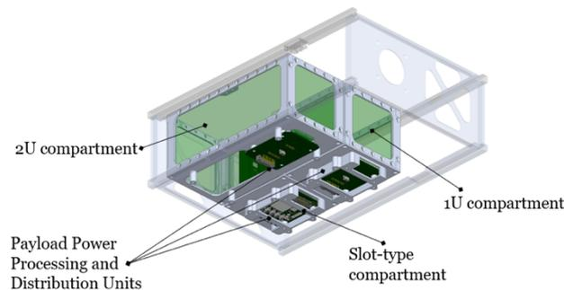
Figure 7: PDU modules distribution in the satellite
