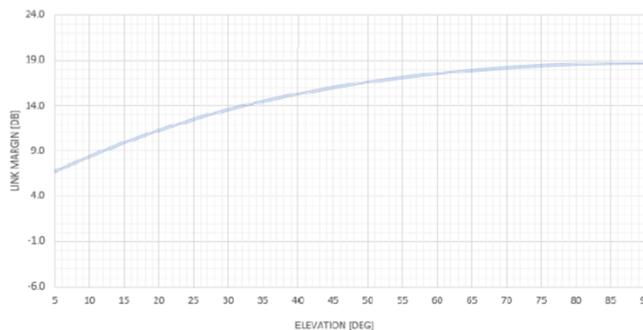
Figure 3: S-band link margin analysis vs elevation
