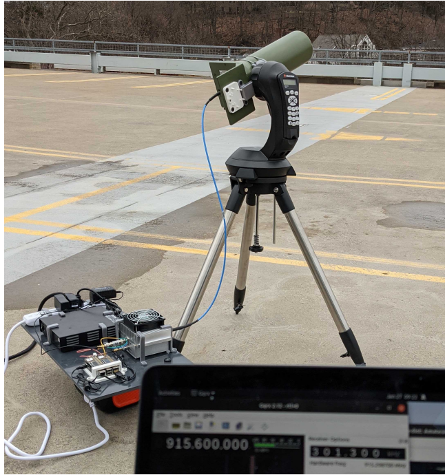
Figure 10. V-R3x mobile ground station. A low-cost amateur telescope go-to mount is used automatically point a 12 dBi gain 915 MHz helical antenna using standard open-source satellite-tracking software. The antenna is connected to a pair of LoRa radios through a low-noise amplifier for receiving and a 50 W power amplifier for transmitting. The entire setup is portable, can be assembled and disassembled in minutes, and can be powered from a lithium-ion battery pack.
