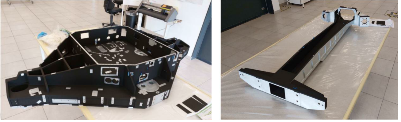
Figure 12. TOB (left) and TMS (right) of the Engineering Model after painting and bakeout, ready for integration. The TOB carries M1 and hosts the instruments in its bay; the TMS connects it to the M2M and M2. The areas left unpainted are the machined interfaces, kept bare for the components mounted on the structure — temperature sensors, accelerometers and, in the instrument bay, the instruments themselves. Image credit: Leonardo S.p.A.
