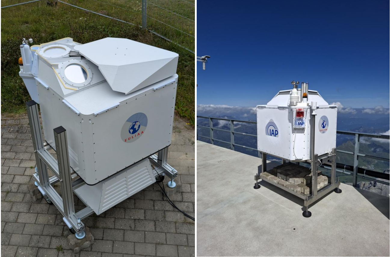
Figure 1. Left panel: EULIAA-IR1 at Kühlungsborn, Germany during early test measurements. The lower part contains the chiller in a separate housing. The upper part of 1\times1\text{ m}^3 contains all hardware of the lidar in a sealed and temperature stabilized 3D-printed housing. Right panel: EULIAA-UV2 on top of the Sphinx station at HFSJG at 3580 m altitude.
