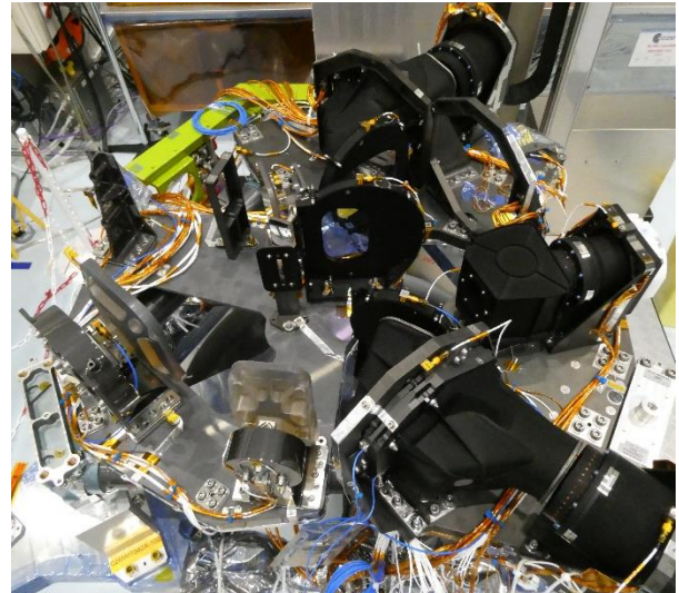
Figure 2. (left) schematic of the CO2I spectrometer assembly, (right) spectrometer bench during its assembling phase.
