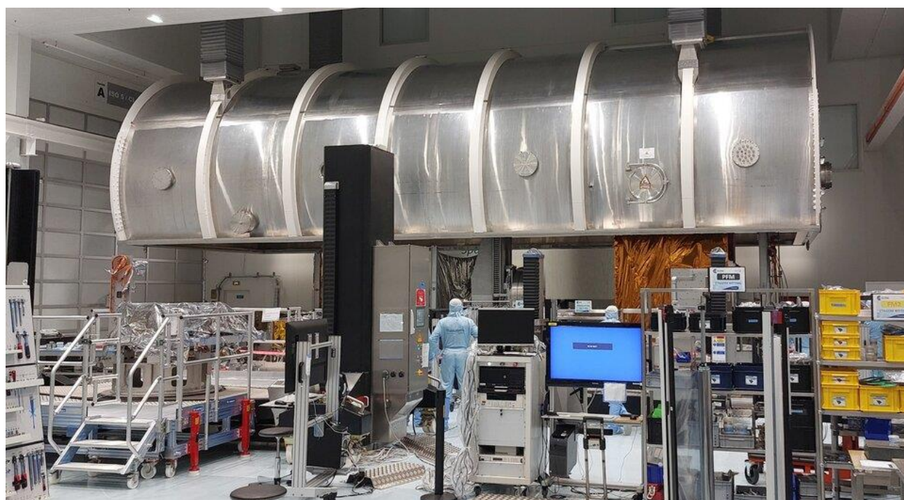
Figure 3. CO2M's spectrometer being sealed within the vacuum chamber
