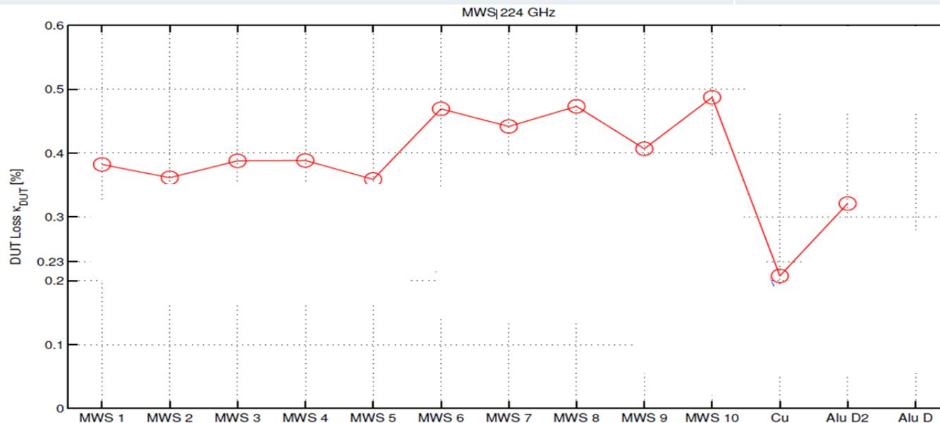
*RF performance for 10 coated samples, 1 Cu reference sample, 2 Al reference sample @ 224 Ghz*
