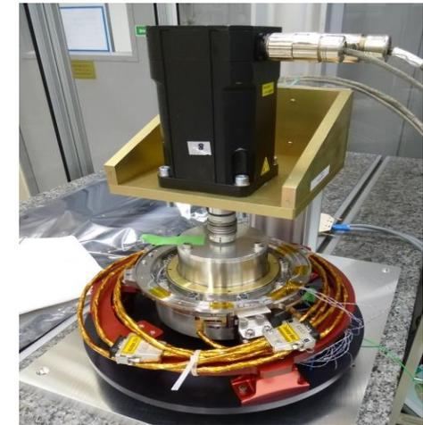
*Bearing Friction Test Setup*
