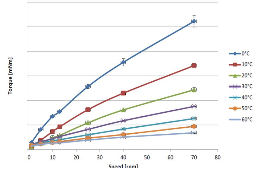
*Derotator LTM Bearing Friction Data*
