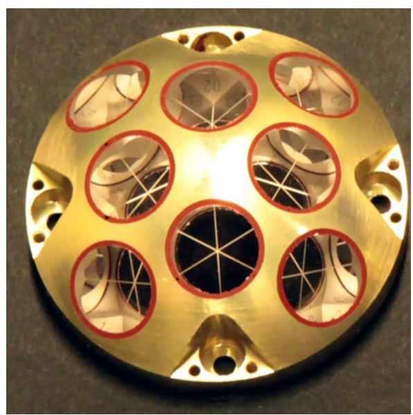
LaRRI for Insight (left) and LaRA for Perseverance (right) microreflectors.
