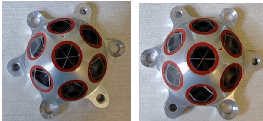
The two MLRH picoreflectors for Hera.
