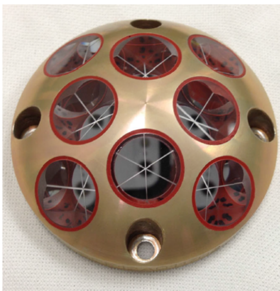
LaRRI for Insight (left) and LaRA for Perseverance (right) microreflectors.
