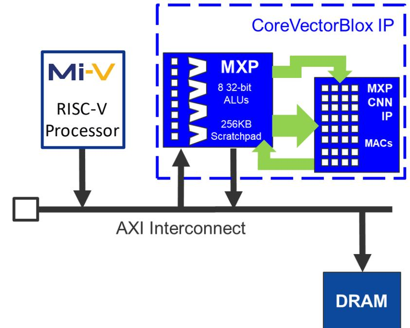
Overlay implementation allows several different networks to run on the same FPGA design without the need to resynthesize
