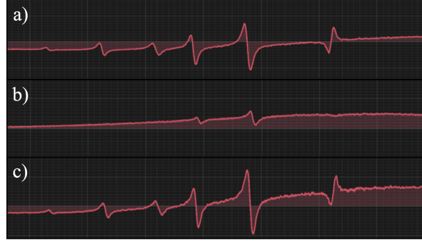
Figure 6. Error signal - double subtraction (example). Polarization subtraction (a), background signal (b), double-compensated signal (c).
