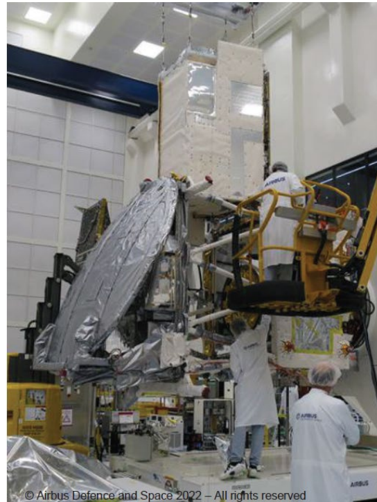
Figure 2. EarthCARE satellite with all instruments integrated, CPR reflector antenna deployed, in Airbus Friedrichshafen cleanroom (left). ATLID integration into the EarthCARE platform (right).
