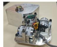
Integrated seismic sensors
