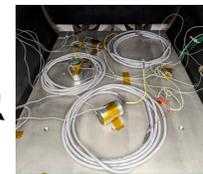
Environment testing of the seismic sensors @ ISAE-SUPAERO
