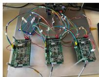
Breadboard of the 3 axis electronics
