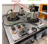
Integrated seismometer performance testbed @ ISAE-SUPAERO
