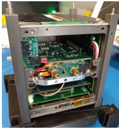
Figure 8. OBDH, EPS and TTC card integration, coaxial cable and interconnect card integration, faceplate integration.
