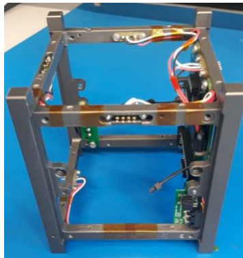
Figure 6. Harness, Motherboard, and Switch PCB Integration
