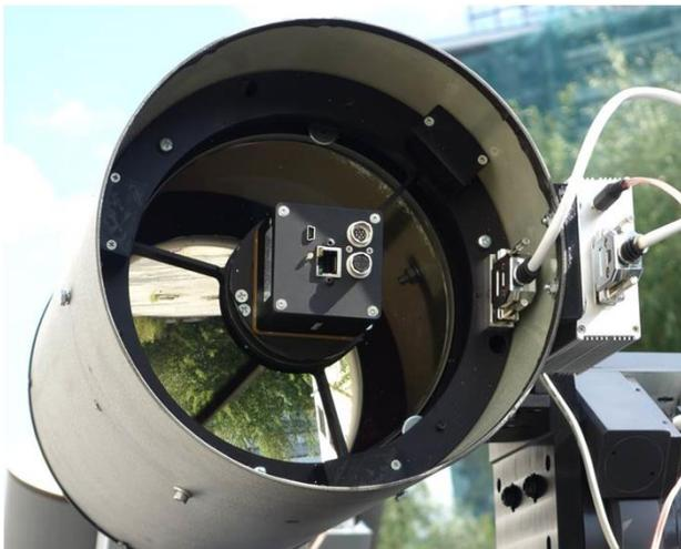
Development of ISON asteroid survey is connected with 40-cm telescope (first in Multa) with FOV 4x5.5 degree and 28-cm telescopes with FOV 6x6 degree (first will be installed in Mexico in this year).
