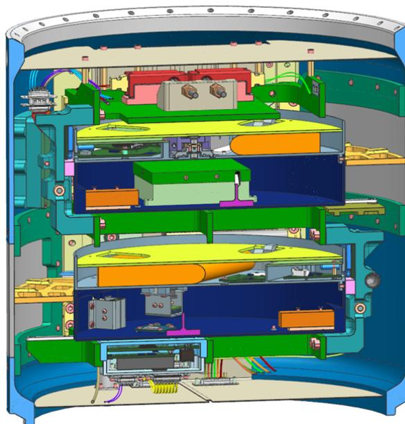
Figure 2: Section of the rocket-mounted unit: ejection mechanism
