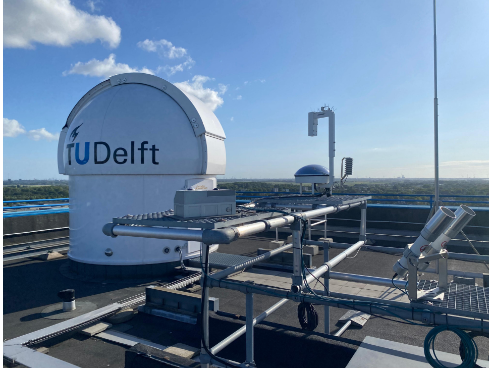
Figure 3: The TU Delft Aerospace Observatory: the Baader Dome housing a 16" Ritchey-Chrétien telescope and turbulence monitoring instruments, including the C-DIMM on the lower right side.
