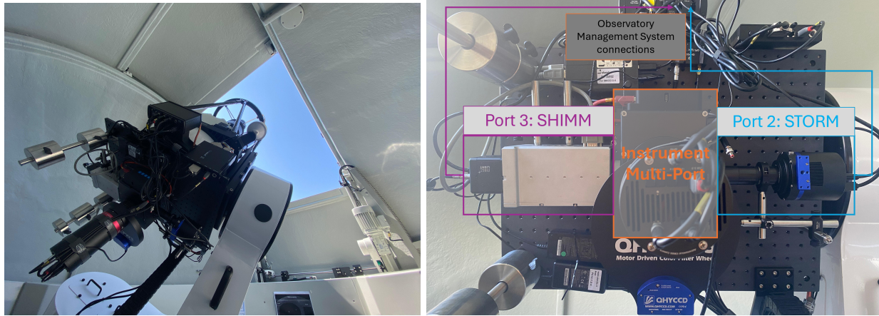
Figure 4: Mounting of the different instruments on the telescope breadboard. The primary mirror is directly behind the breadboard and the IMP redirects the light towards either Port 2 or Port 3. Each instrument is connected to a power and data hub which is directly linked to the observatory computer.
