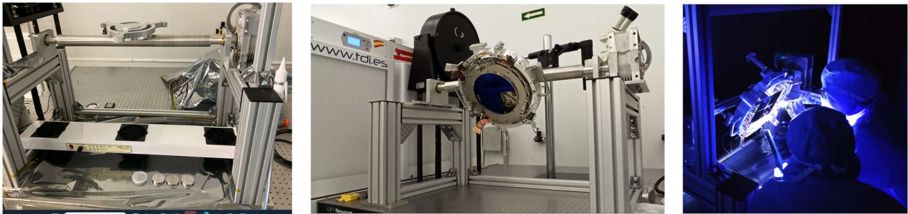
Figure 7. From left to right: Flipping jig; FPA mounted on flipping jig ambient light on; FPA mounted on flipping jig ambient light off.
