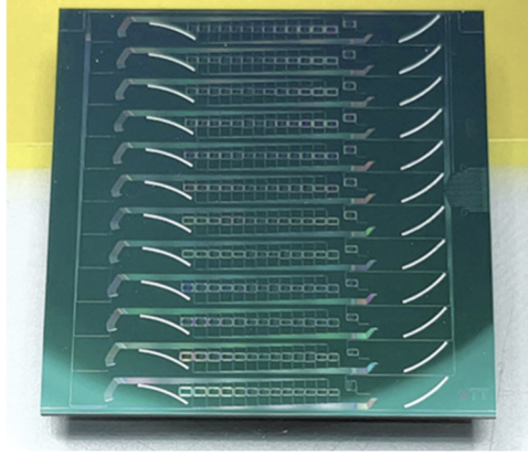
Figure 2. Photograph of the fabricated ACTA-UHTS beamformer photonic chip
