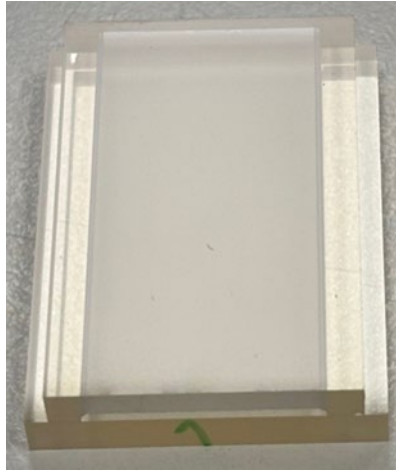
Figure 5: Tensile test sample with two fused 3 mm x 40 mm sized ribs.
