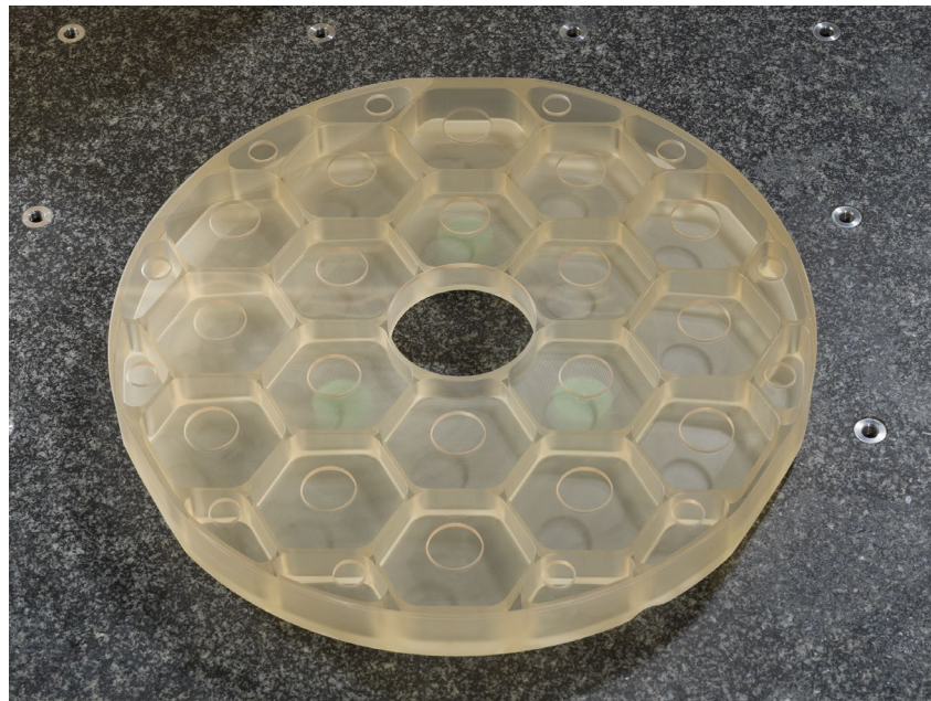
Figure 3: 480 mm demonstrator with 4 mm rib thickness [1].
