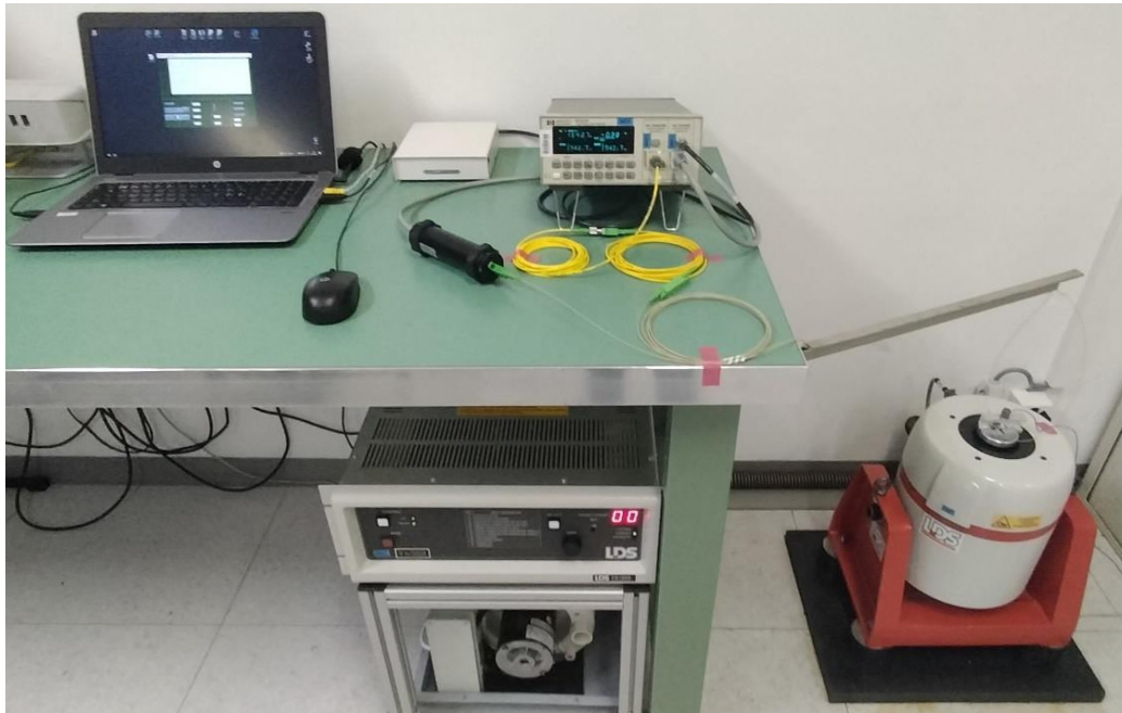
Figure 3. Mechanical test arrangement used during Phase 2 for random vibration and mechanical shock. Source: Diamond SA internal
