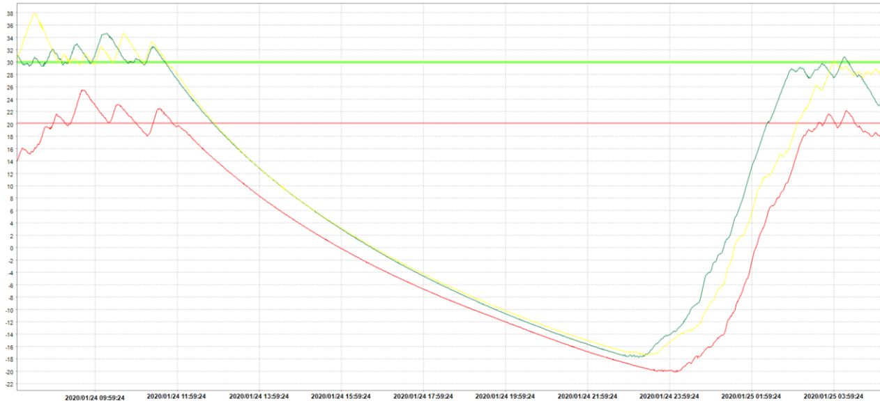
Figure 6: Comparison of the effect of “End of day” heating on battery temperature
