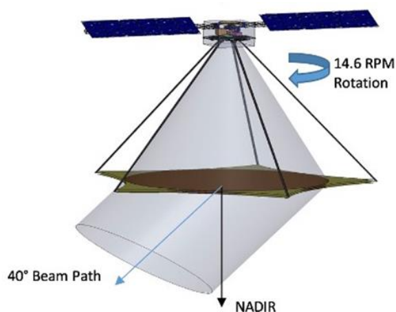
Figure 3: Illustration of the GLOWS antenna beam steering provided by its phase-shifting lens antenna.
