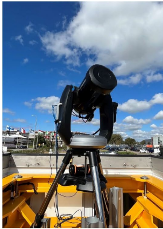
Figure 8. Left: the Portable Optical Ground Station (POGS) at ESTEC. Right: Active illumination preliminary optical design schematic of CIICLOPE system.
