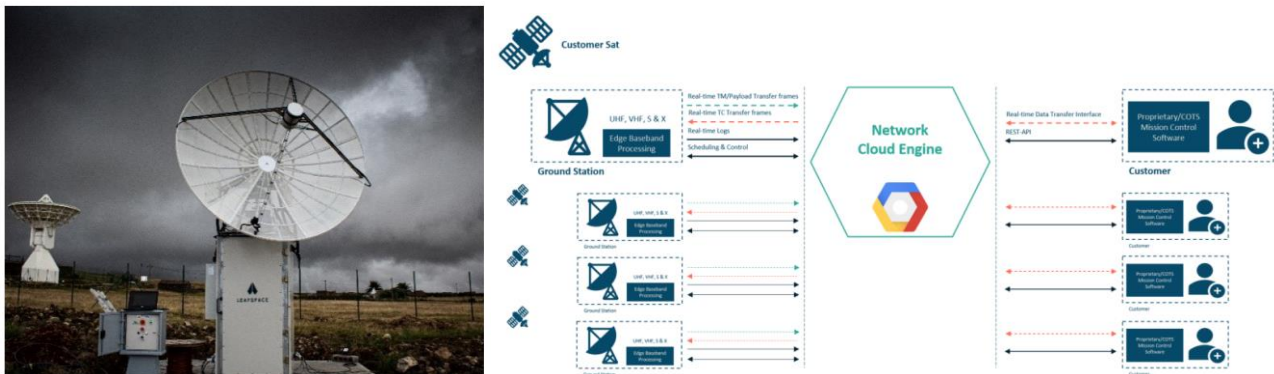
Figure 4. LeafSpace ground stations picture and functional diagram (credit by LeafSpace).
