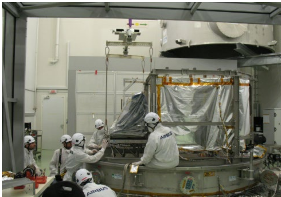
Figure 33. AIT activity in the AIRBUS GAIA chamber for the co-alignment of the AOB/DBS2/POB and its verification in TVAC
