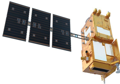
Figure 1. General view of the LSTM satellite. The payload composes the lower module on this picture
