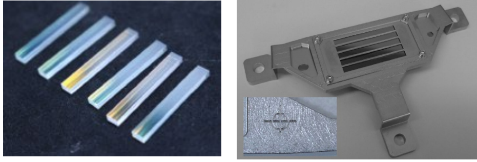
Figure 5. VNIRSWIR stripe filters (left) (courtesy of OBJ) and TIR detector plane filters assembly (right) (courtesy of the University of Oxford)
