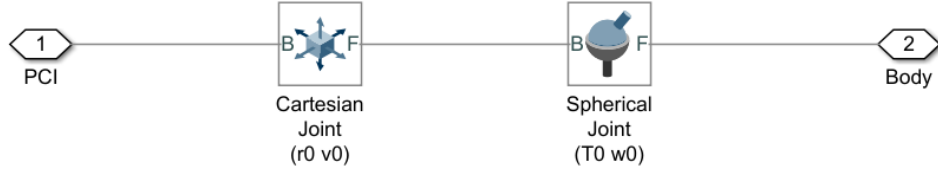
Figure 4: Implementation of launch vehicle dynamics using Cartesian- and Spherical Joints
