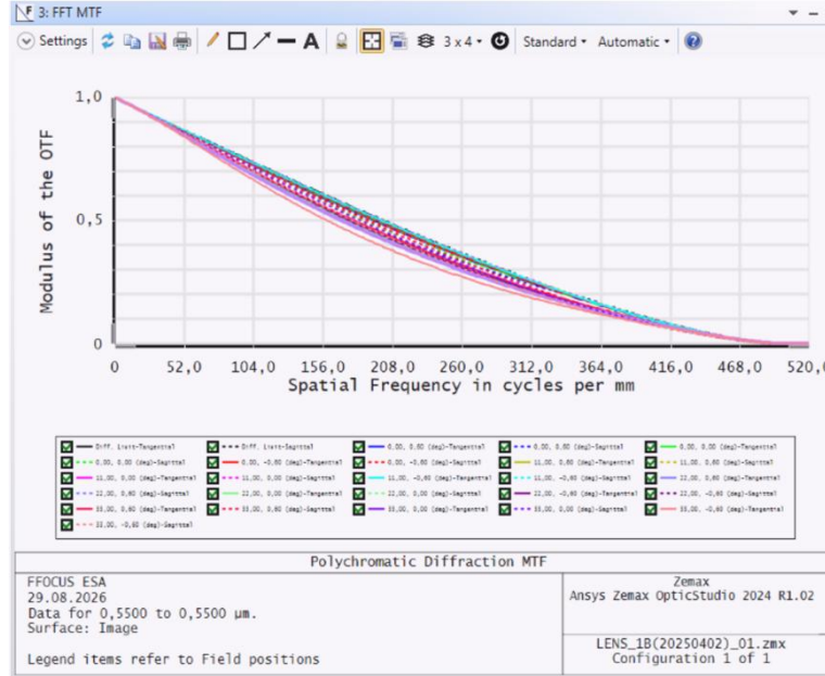
Figure 3: MTF of the nominal design of the telescope.
