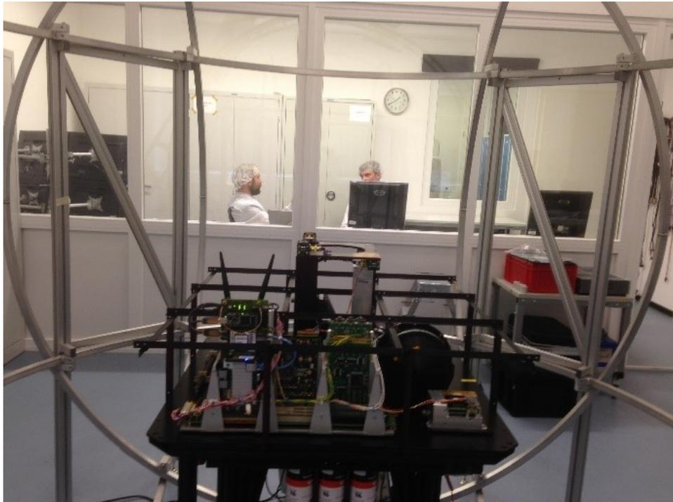
Figure 2 The equipped BIROS EM-ACS test stand in the clean room of Astro Feinwerktechnik Adlershof GmbH (2015)
