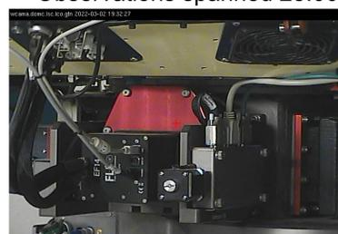
A FLI instrument on the side port of one of the LCO 1m telescopes. The FLI imagers, are normally used as autoguiders with the Sinistro imagers (see right), can also be operated as fast frame rate cameras.
