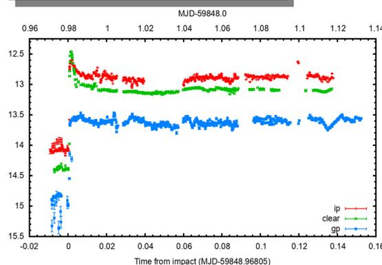
Three color lightcurves (SDSS g' (blue points) & i' (red points) along with a 400-1200nm bandpass clear filter (green points)) of Didymos from the LCO 1m+FLI instruments at SAAO during the DART impact. Cameras. There is considerable chromaticity in the ejecta with the red (i') and clear filter showing a large brightening ( $\sim 2$  mags) and then a rapid decay while the bluest (g') data showed only a steady  $\sim 1.5$ mag increase in brightness.
