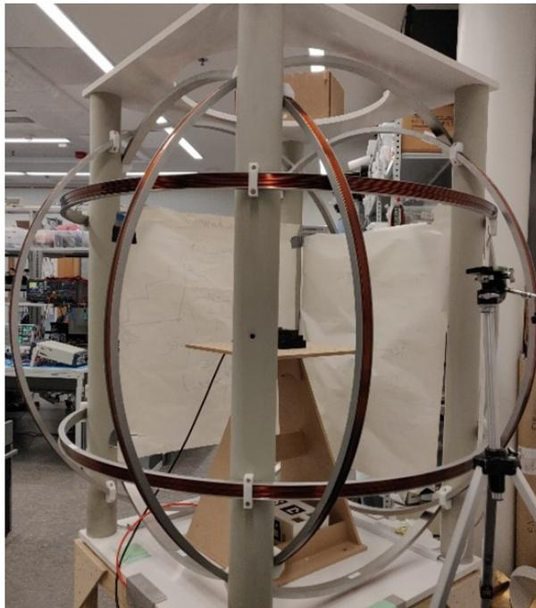
Figure 3: Helmholtz coil system used to calibrate MATTI. The three-axis coil system is located in a laboratory environment and surrounded by other electronics causing magnetic interference, especially at the mains frequency of 50 Hz. The black object in the middle of the coils is the reference fluxgate magnetometer used for calibration and characterization. Image courtesy of Aalto University.
