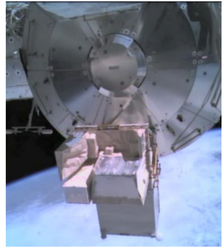
Fig. 1: ACES installed on the ISS, at the external payload facility of the Columbus module (Credits: ESA-NASA).
