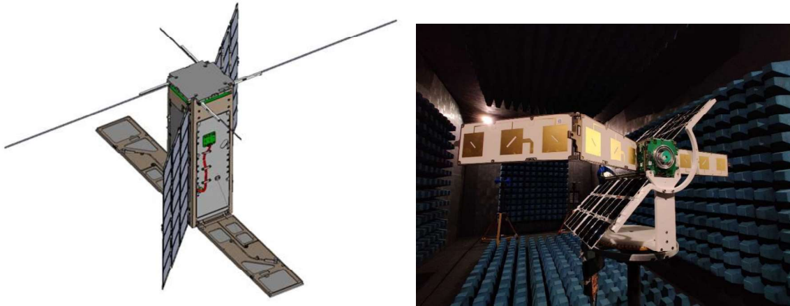
Figure 2 - GNSS-R satellite. (Left) Physical location of the POD antenna is on the very top of the satellite while the GNSS-R antennas are on the downward facing panels at the bottom. (Right) GNSS-R satellite in testing chamber placed here for visualization purposes.
