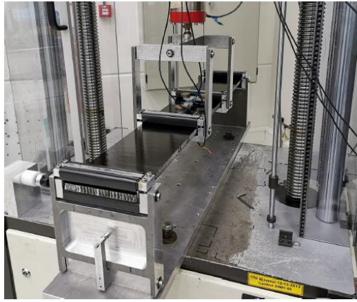
Figure 9: 4-point bending substrate testing
