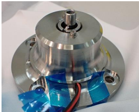
Figure 4: Central hold-down and release mechanism
