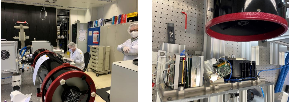
Figure 9. Test setup for adjusting the focus in lab
