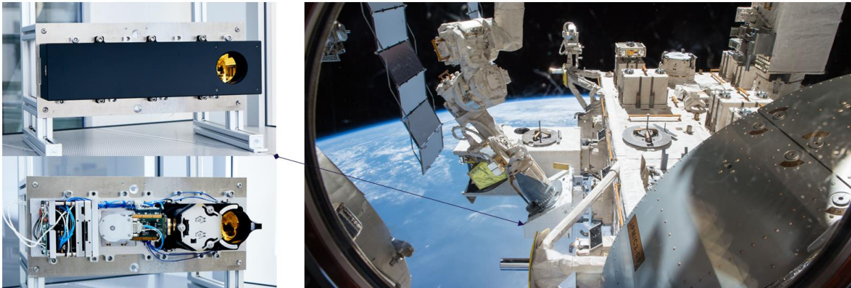
Figure 1. Upper Left: LisR instrument with its black painted cover. Bottom right: LisR instrument without cover. The different subsystems, like the data and power processing unit, the TIR detector and the telescope are visible. Right: Location of LisR on the NanoRacks Experimental Platform NREP.
