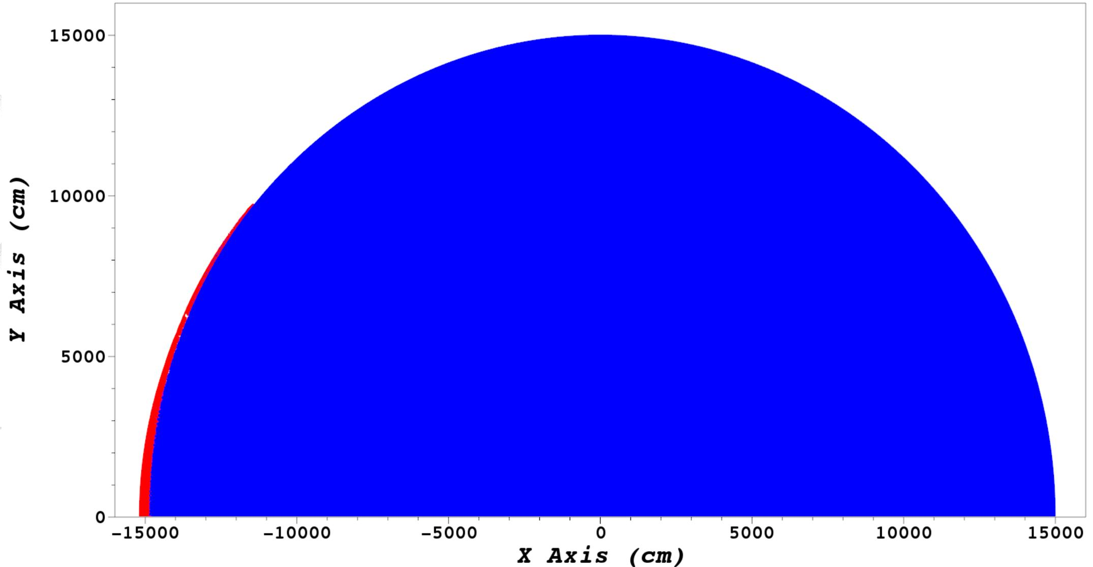
**Red = blow-off = fragments that are melted and traveling faster than escape velocity.** 16
