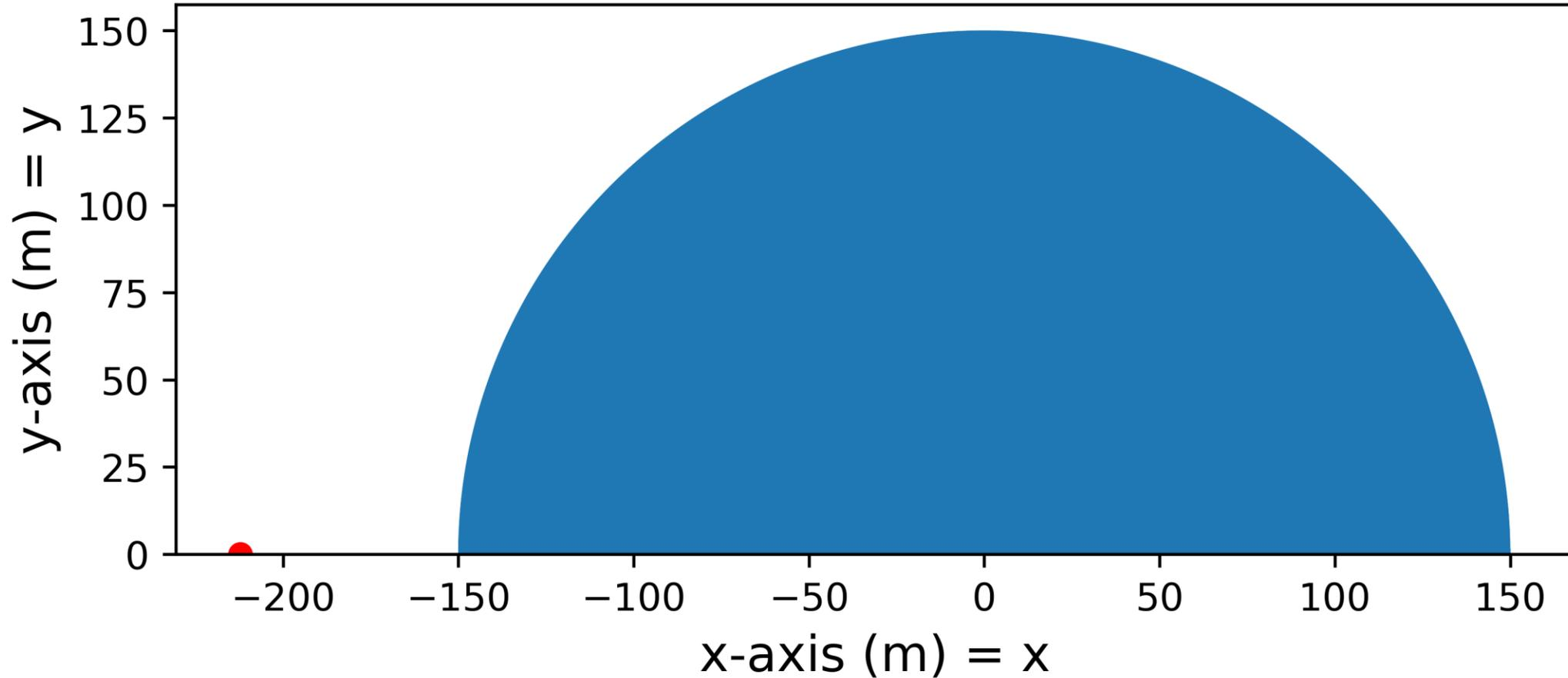
**2-D axisymmetric geometry allowed for a semi-circular asteroid model, saving computational resources and achieving sufficient mesh resolution.**
