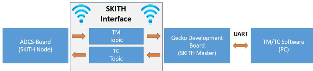
**Fig. 8:** Interface between the adcs board and the TM/TC development software
