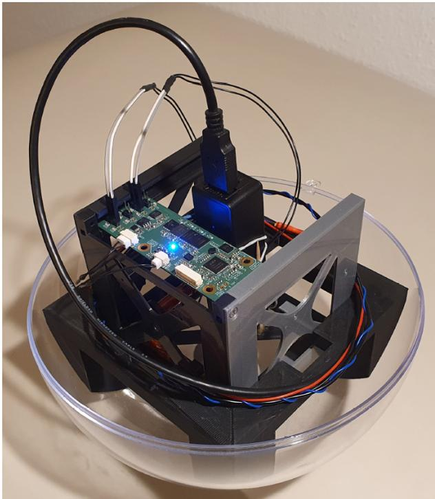
(a) ADCS test-box using external power supply
