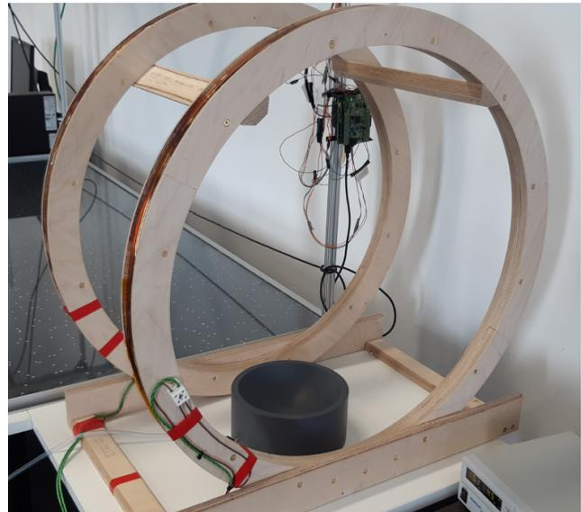
(b) Air-bearing table and helmholtz coils test setup
