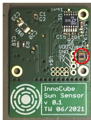
(b) Sun Sensor PCB (optical sensor marked red)
