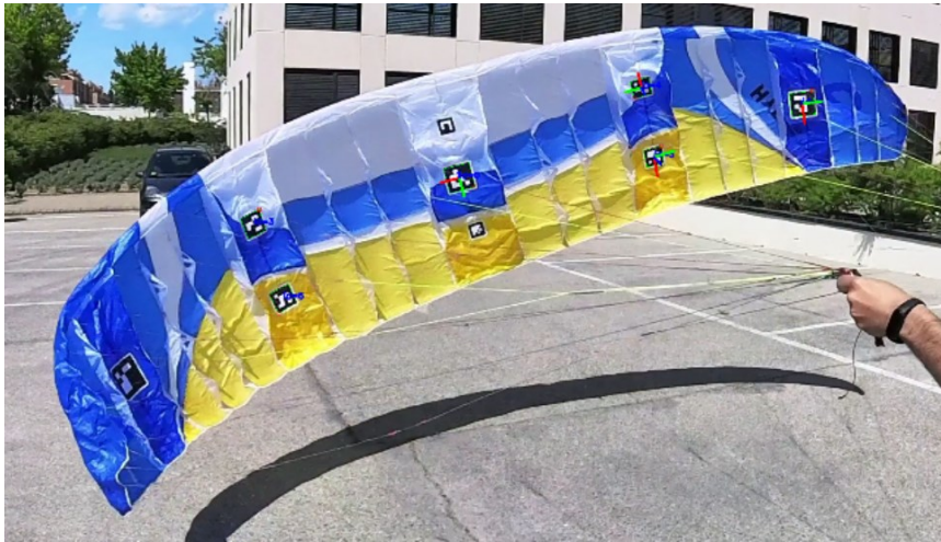
Figure 5-2: Parafoil Attitude Estimation with ArUco Markers
