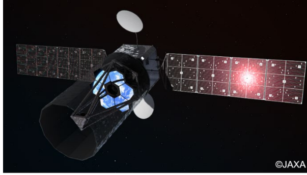
Figure 1. Conceptual image of a GEO optical satellite for Earth observation with a segmented mirror telescope system.
