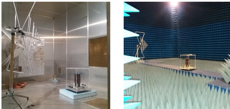
Figure 1 : The reverberation (left) and the anechoic (right) rooms with the 3U Cubesat test platform
