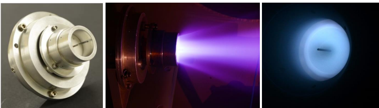
Figure 4 : Left, the microwave electrical thruster, ECRA. Middle, the 30 W version. Right, the 200 W version
