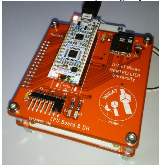
Figure 3. Assembly of EPS and CPU boards
