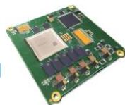
This modular system is based on a latest generation multiprocessor System-on-Chip, robustified by rad-hard elements to offer an unprecedented processing power and efficiency on your mission. It allows further system miniaturization, system performance enhancement and in-orbit reconfigurability.
