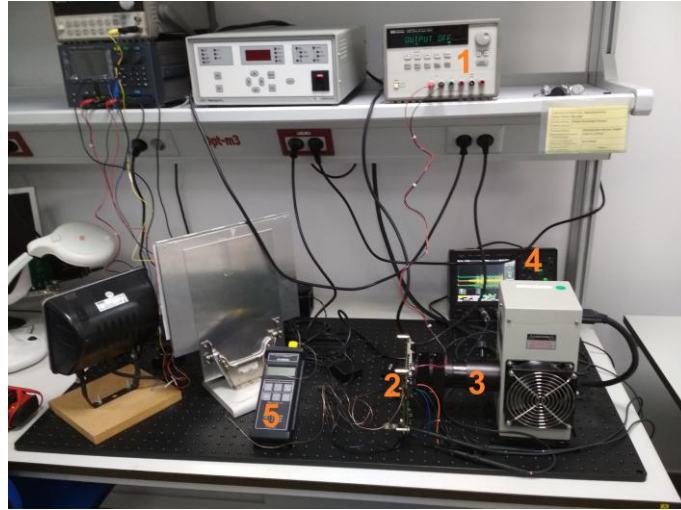
Figure 2. Setup for electro-optical measurements: 1 – power supply, 2 – motherboard with DUT mounted on top, 3 – light source with corresponding neutral filters for illumination level control, 4 – oscilloscope, 5 – thermometer.
