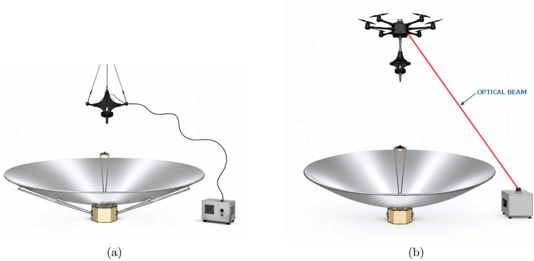
Figure 2. Conceptual illustration of phase-reference distribution in antenna measurement configurations: wired link in a gondola-based setup (left) and optical wireless link in a UAV-based setup (right).
