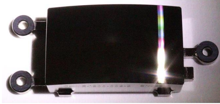
Figure 2 Photograph of one of the CHIME diffraction gratings (before coating)
