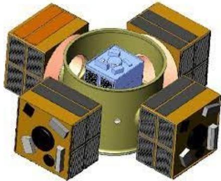
← Internal ESPA ring hosts all MUFN power and avionics systems (option to stack multiple rings adds modularity to design)
