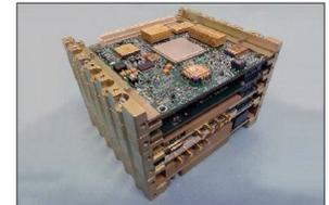
Figure 1: Illustration of the Iris V2 radio (image credit: JPL)
