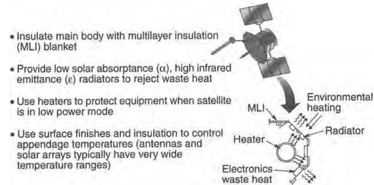
Fig. 3.2. Three-axis-satellite thermal control.
