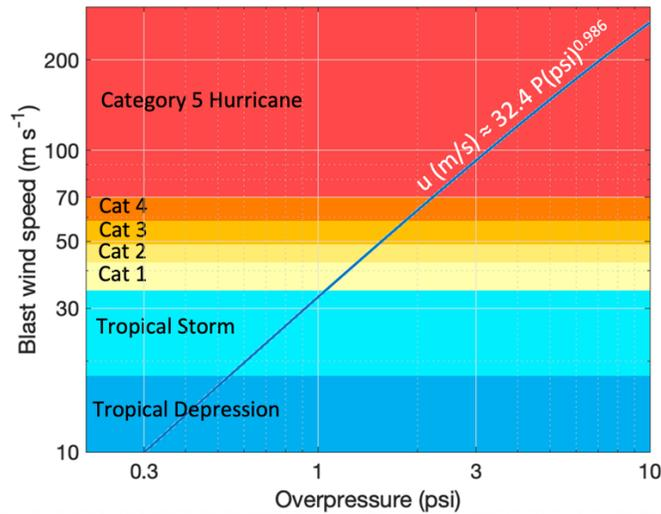
Figure 13: Wind speed behind a blast wave including a ground reflection. Assuming buildings suffer damage due to wind speeds sustained over a few seconds it also gives the equivalency of storm winds and blast waves. This will allow risk estimates to be calculated at both high and low overpressures when taking appropriate shelter.
