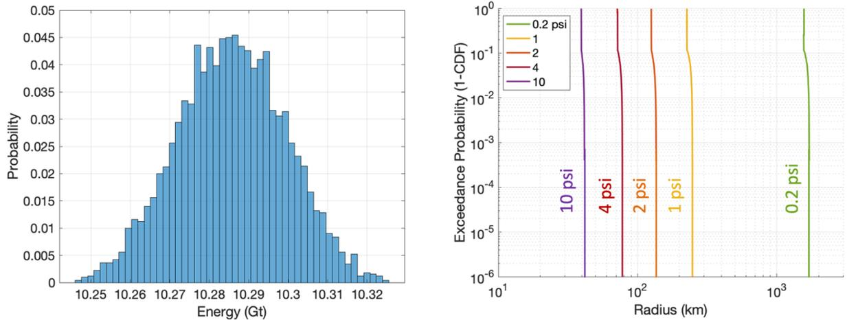
Figure 21: Rendezvous mission very precisely determines the mass, velocity, and hence impact energy of the asteroid. The large mass means the asteroid hits the ground mostly intact so the predicted blast radii are also very precise. Model uncertainties (not accounted for here) will be greater than the uncertainties in the asteroid.
