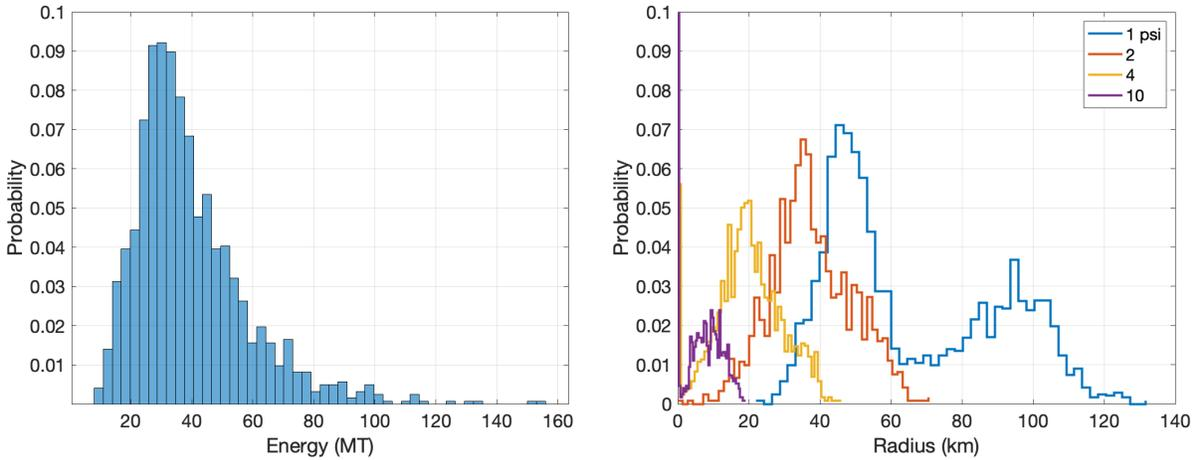
Figure 16. Asteroid impact energy follows a distribution due to uncertainties on composition, density, and porosity, despite the diameter being well constrained from radar measurements. Distance at which a given pressure level is felt from the blast varies additionally with uncertainties on strength and height of burst.
