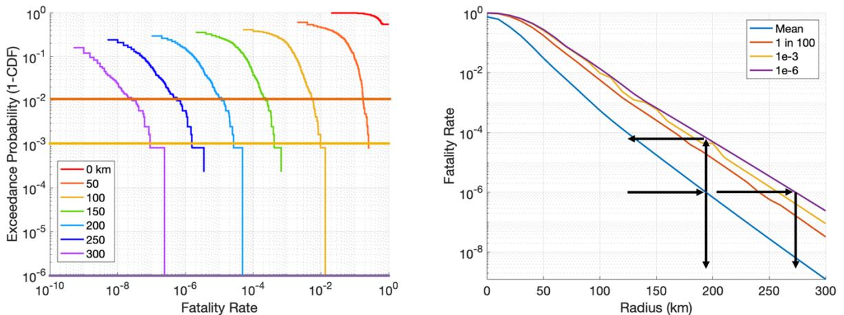
Figure 17. Probability of exceeding a given fatality rate vs distance. The closer to the blast the more likely a higher fatality rate is. The mean value for the 1 in a million fatality rate is at about 200 km, but there is a  $10^{-3}$  (1 in 1000) chance of the fatality rate at that distance actually being  $10^{-4}$  (1 in 10 000) and the 1 in million rate actually being at 270 km distance.
