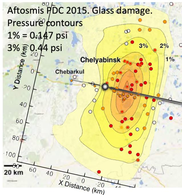
Figure 14. Estimated blast peak overpressure and map of broken windows. The peak pressure required to break windows is about 0.1 – 0.2 psi. (Aftosmis, et al., 2016)
