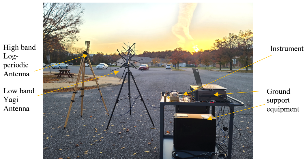
Figure 7. Live sky instrument test setup.
